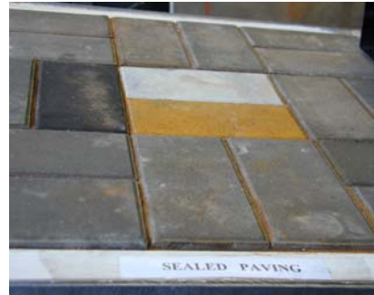
FIGURE 9 – Sealed IPS units after test
